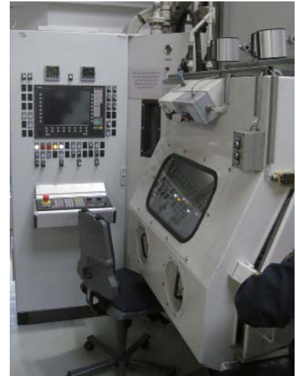
CNC control-cabinet of wet blasting machine
